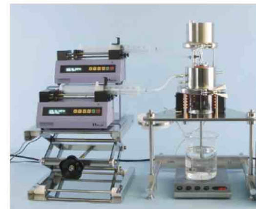
Var D Generation II (Nisco, CH) - electromagnetically driven generator
