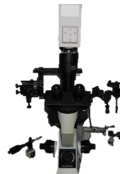
Olympus CK 40 inverted microscope system with micromanipulator NARISHIGE TM-50B
