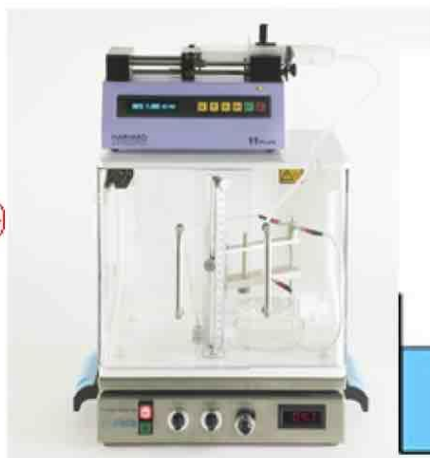
Var V1 (Nisco, CH) - electrostatic capsule generator
